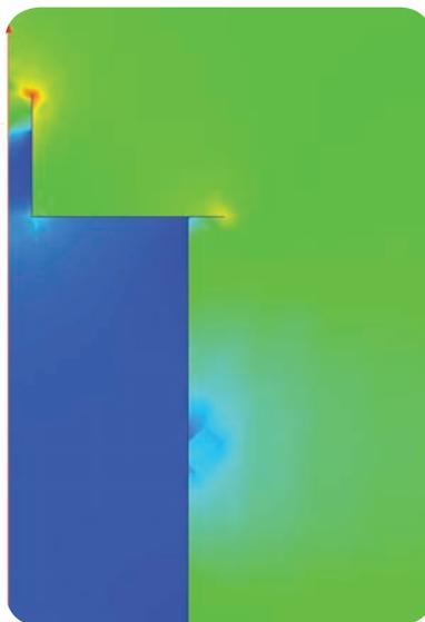
▲ ANSYS Maxwell 2-D simulation identifies small amounts of leakage through shielding.
