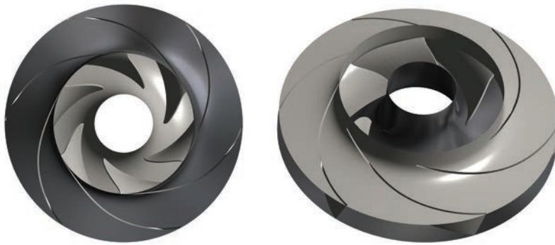
▲ Parametric model of the impeller used to define hydraulic geometry
