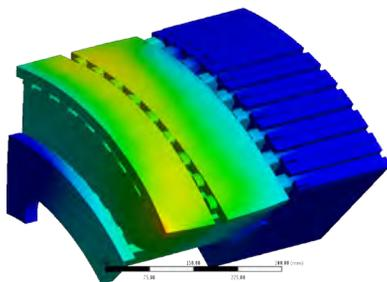
**Banding radial displacement evaluation with ANSYS Mechanical**
