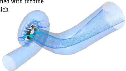
Complete model of Francis turbine simulated with ANSYS CFX
