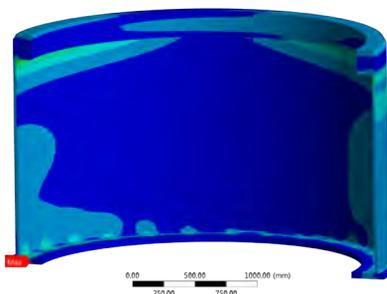
◀ Nacelle tower-top adapter (left). Evaluation of neck stress and welding point (right).
