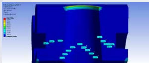
▲ Another view of temperature distribution on final design shows lower temperatures and more even temperature distribution.
