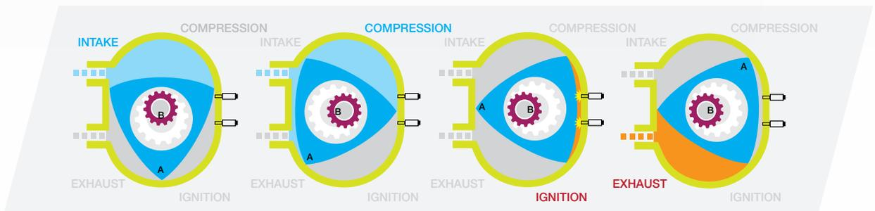
▲ Diagram of the four-stroke cycle of a generic rotary engine. Courtesy: Y\_tambe's file. Permission =GFDL
