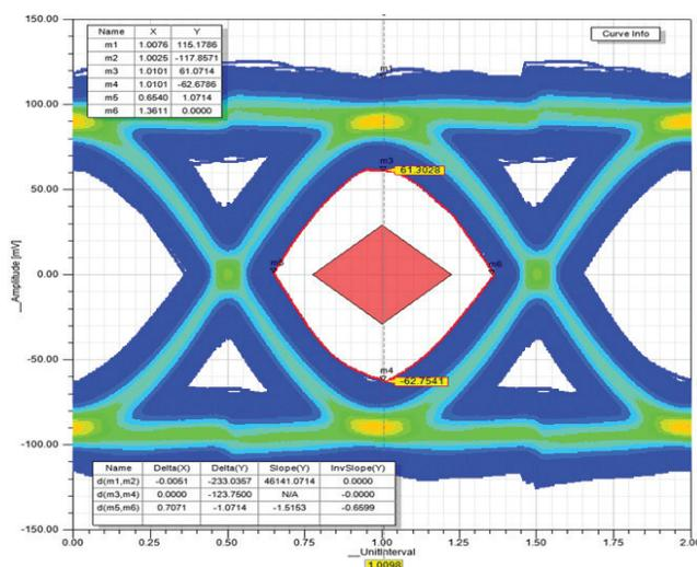
▲ Eye mask simulation shows signal after RX equalizer and DFE.
