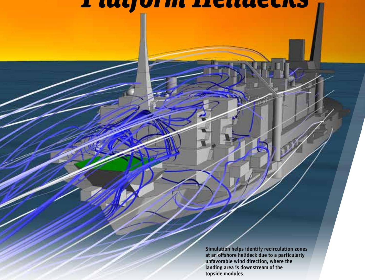
Simulation helps identify recirculation zones at an offshore helideck due to a particularly unfavorable wind direction, where the landing area is downstream of the topside modules.
