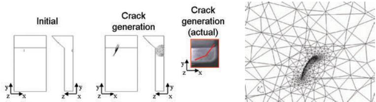
▲ Crack growth analysis allows DENSO to predict when failure might occur. This helps to ensure product reliability by visualizing the stress distribution based on crack profile changes.
