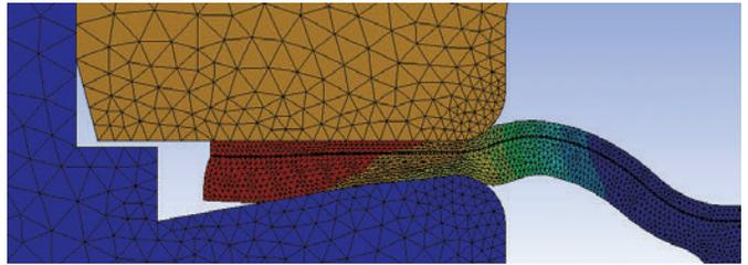
▲ Using large deformation analysis allows the DENSO team to predict strength and the shape profile. With some compressions at more than 50 percent of the original thickness, structural simulation helps the company to ensure product reliability.
