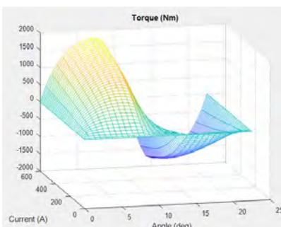
3D map of produced torque as a function of current load and rotor position
