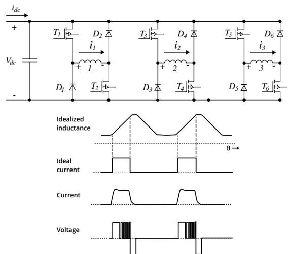
Asymmetric bridge converter circuit diagram (top) and resulting SRM waveforms
