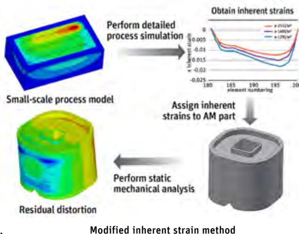
But topology optimization typically requires running hundreds of simulation iterations in a batch, so performing the full thermomechanical simulation required to simulate metal additive manufacturing would take too long to be relevant in a real-world engineering environment.
