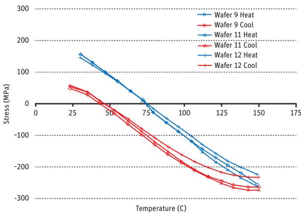
▲ Thermal cycling caused a 100 MPa change in residual stress due to plastic deformation of the metal film.
