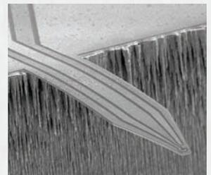
▲ A MEMS cantilever sensor designed and prototyped by AMFitzgerald
