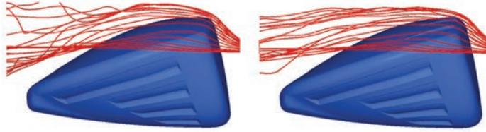
▲ CFD simulation of clubheads without (left) and with (right) turbulators shows how the new design delays flow separation and reduces drag.
