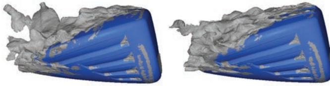
▲ Side view of simulation without (left) and with (right) turbulators shows that wake is smaller with turbulators.
