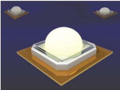
▲ DuPont CoolLam® thermal substrate improves thermal management of LEDs.
