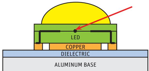
▲ CoolLam® thermal substrates consist of copper foil, polyimide dielectric and aluminum base. The arrow shows the center of the thermal pad, which cannot be measured under operating conditions.
