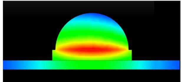
▲ Simulation results show temperature plotted on LED, thermal substrate and board.
