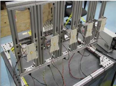
▲ Test setup in laboratory with yellow LED mounted on thermal substrate hidden behind LED and thermal substrate mounted on gray board
