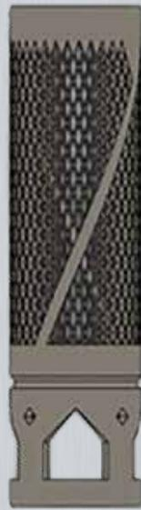
CAD model of redesigned part with supports incorporated into mesh
