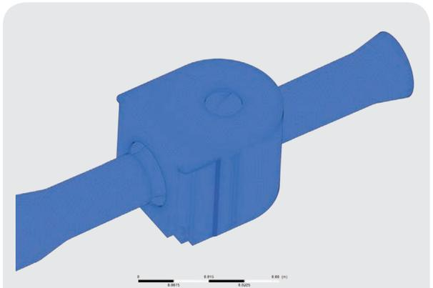
Overall volume mesh for CFD simulation
