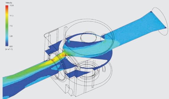
Velocity contour plot of valve at partially opened position
