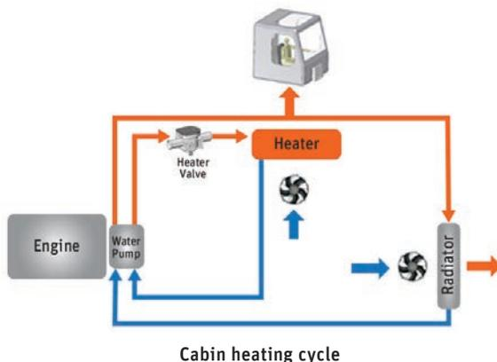
and efficiently. MCC engineers developed an optimized design for the valve geometry that maximized its ability to precisely control the volume of coolant that flows through the valve at each position of the valve’s knob to improve cabin heat control.
