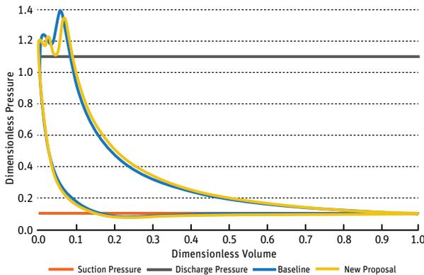
▲ Pressure-volume chart quantifies losses on suction and discharge sides of compressor.
