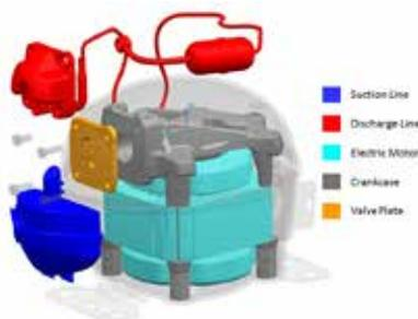
▲ Diagram of compressor parts
