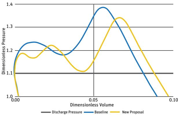
▲ Discharge losses were reduced in the new design (blue) versus the previous generation (yellow).
