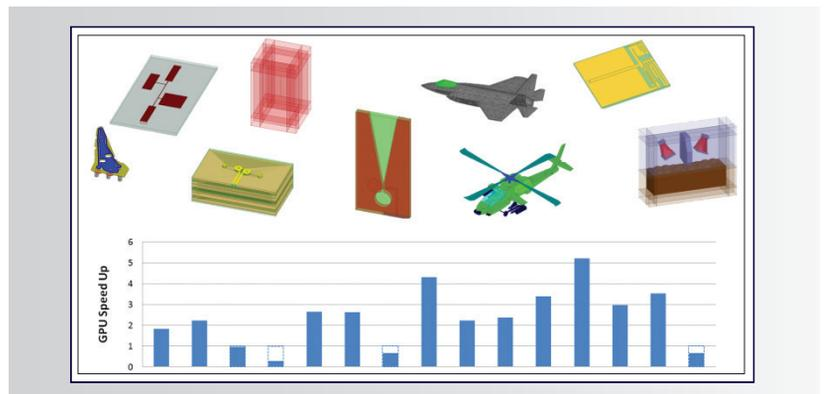
▲ ANSYS HFSS transient benchmarks on one NVIDIA Tesla K20 compared with eight cores of Intel Xeon X5675. Only nine of the 15 benchmark structures are shown in the figure. Dotted lines indicate cases in which the GPU did not provide speedup and CPUs were automatically used.
