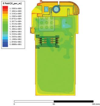
▲ A smartphone for transient field analysis on CPU, memory, GPS and Bluetooth ports due to power surge during battery charging. The model was discretized into 1,093,376 tetrahedrons.
