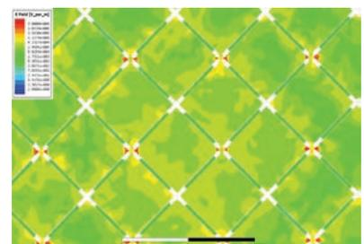
▲ Strong electric fields (red) on the bridges between sensor pads of the touch screen of a handheld device cause dielectric breakdown of indium-tin-oxide (ITO) thin films.
