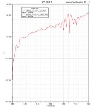
▲ Three patch antennas placed on the tail of a helicopter (top) and their S-parameters from DC to 1.2 GHz (S11 bottom left, S12 and S13 bottom right). The length, height and wingspan of the helicopter are 17.73 meters, 4.05 meters and 5.23 meters, respectively. The model was discretized into 549,247 tetrahedrons.
