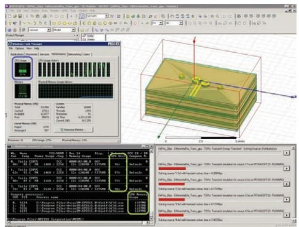
▲ Network analysis of differential stacked vias on four GPUs. Simulation jobs are run in parallel as shown by the progress bars and NVIDIA System Management Interface (nvidia-smi). The model was discretized into 68,401 tetrahedrons.
