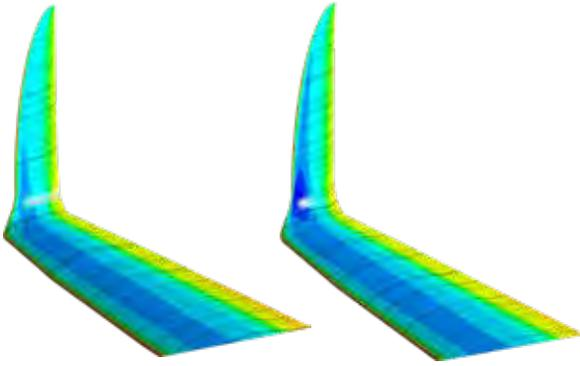
ANSYS Fluent CFD revealed unfavorable pressure peaks in the area of the wing–winglet junction, which was originally designed with classical aerodynamic tools. After design iteration with Fluent, it was possible to alleviate this problem and gain some aerodynamic efficiency.
