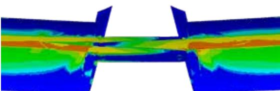
Safety factors for the carbon fiber–reinforced plastics structure in the area of inner-wing junction were analyzed with ANSYS Composite PrepPost.
