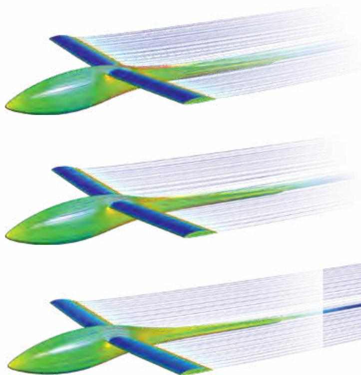
Configuration investigated for the wing-fuselage junction including a high-wing position (top) to a mid-wing position (bottom). Calculations revealed minimum drag for the mid-wing position, especially at high airspeeds.
