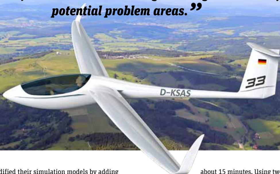
iteratively modified their simulation models by adding more plies or changing already existing ply properties such as ply extent, fiber orientation or materials at high load points to eliminate any weak points in the design.
