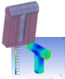
PADT staff used ANSYS Additive Print to design the supports. The software predicted a distortion of 0.4 mm vs. the 3.0 mm with the standard supports.
