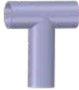
The team decided to really put ANSYS Additive Print to the test by simulating and manufacturing a T-tube model that PADT has been making for decades, to test support structures and accuracy for plastic and metal 3D printing.
