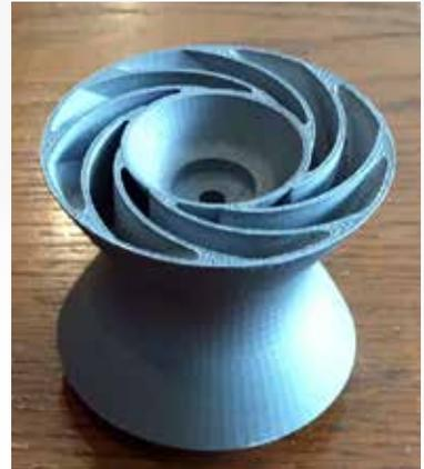
**ANSYS Additive Print confirmed that no additional supports were required for this part for a small gas turbine. The manufactured item verified the correctness of the part.**
