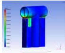
After generating supports using PADT's standard 3D printing pre-processing tool, the team performed a quick assumed strain analysis in Additive Print and determined that the model was not being held properly. The first layers at the bottom of the horizontal tube distort significantly so that if the part had been printed, the layers would probably pull off the support and crash the machine.
