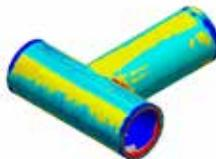
When the scan results were compared to the final geometry, it was revealed that the surface roughness from the support material removal is the cause of most of the deviation, not thermal distortion. In areas away from the surface roughness of the support attachments, the distortion is only about 0.13 mm, showing that the optimized supports and distortion compensation from ANSYS Additive Print produced a final printed part well within acceptable tolerances.
