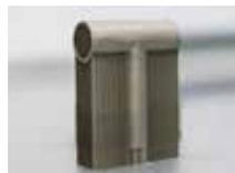
The part (including the supports) was printed in 17-4PH stainless steel on a Concept Laser MLab laser powder bed fusion system.
