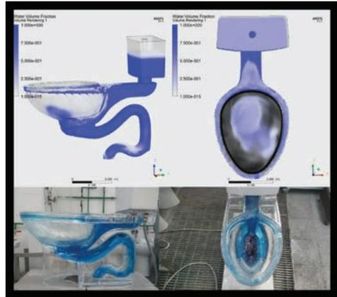
By first constructing a physical toilet model, Roca engineers were able to compare and verify the results of their early simulations — giving them the confidence they needed to eliminate some physical testing.
