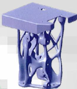
CAD model of sun assembly sensor support
