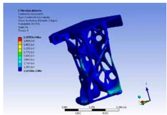
Von Mises stress plot created by finite element analysis of model based on CT scanning of physical part in ANSYS software
