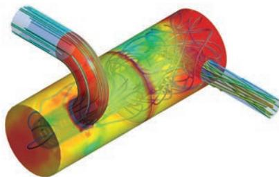
▲ Flow field streamlines and temperature distribution inside muffler displaying fluid streamlines and temperature contours
