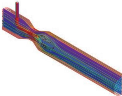
▲ Flow field streamlines and temperature distribution inside venturi-type aspirator
