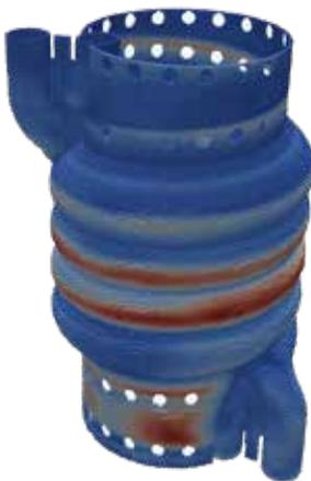
ANSYS Additive Print predicts displacement for a heat exchanger. Courtesy Additive Industries.
