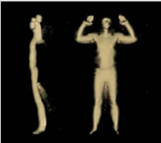
Use of 5 GHz bandwidth and 60-degree beamwidth showed impact of reduced depth resolution on image quality.
