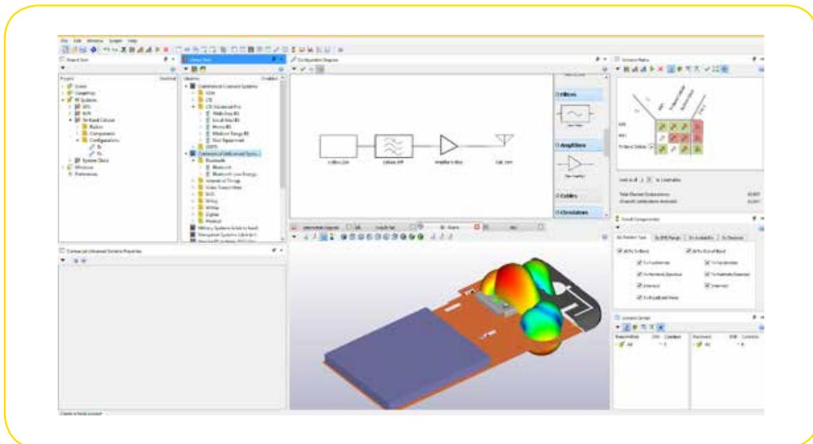
ANSYS EMIT is a unique RF interference tool that can evaluate system performance in complex RF environments. The EMIT desktop shown here includes the HFSS model, radio circuits and a unique scenario matrix in the upper right corner. The red squares in the scenario matrix indicate several RFI issues that must be addressed, while green squares show no problems present.
