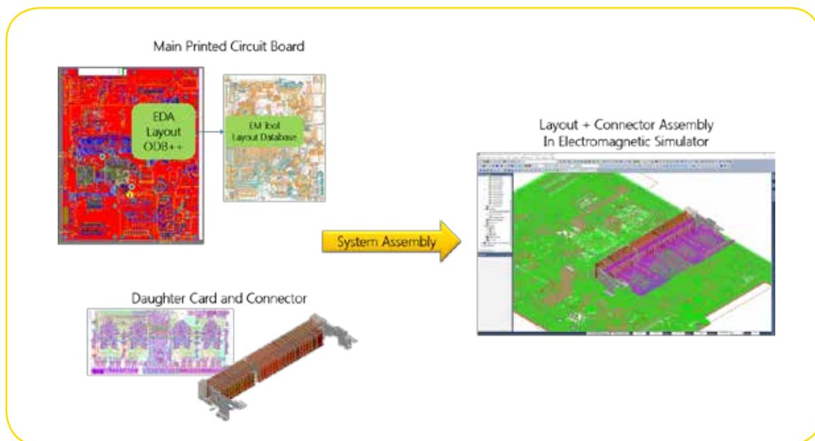
Three-dimensional layout with integrated system assembly for a laptop computer that combines a main printed circuit board layout coupled with an edge connector and a daughter card
