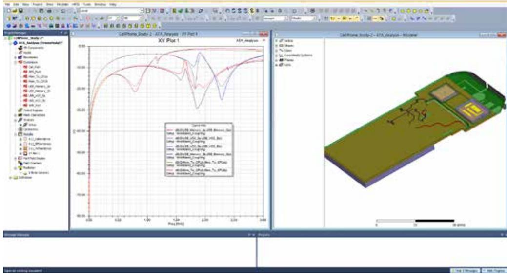
Simulation of a smartphone in ANSYS HFSS. Coupling among antennas and components across the frequency spectrum is shown on the left and the 3-D geometry is shown on the right. HFSS predicts the installed antenna performance, and coupling among antennas and signals on the PCB, across a broad range of frequencies.
