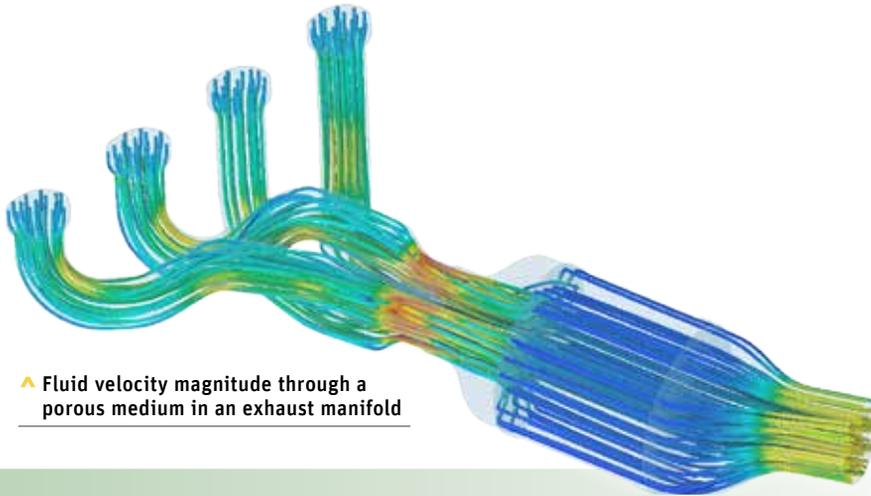
▲ Fluid velocity magnitude through a porous medium in an exhaust manifold
