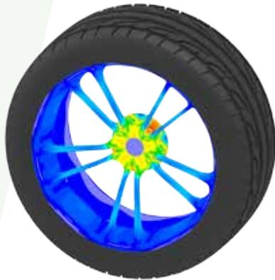
▲ Equivalent stress from sequential bolt pre-tension simulation of an automobile rim
