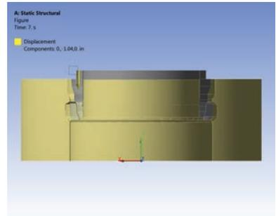
Maximum ring expansion force was retrieved by applying displacement boundary condition to expand the ring.
