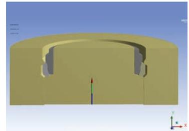
Reaction force to match the pressure rating of the wellhead was generated by applying displacement boundary to move the ring upward.
