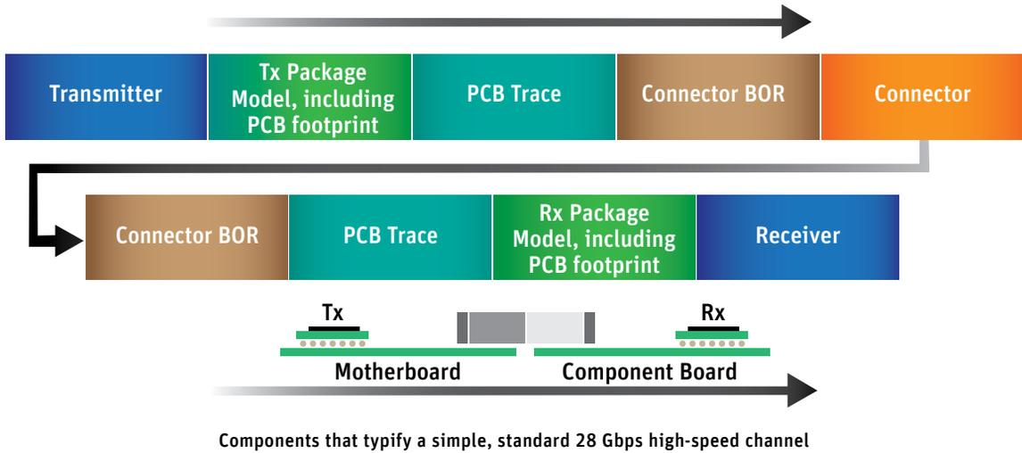
crosstalk and impedance must be considered. PCB design decisions include placement, routing, material/laminate selection, trace lengths and impedance matching — all of which can enhance or adversely affect the performance of the high-speed serial channel. The breakout region (BOR) of PCB traces from the connector is often overlooked, yet it can break a design.
