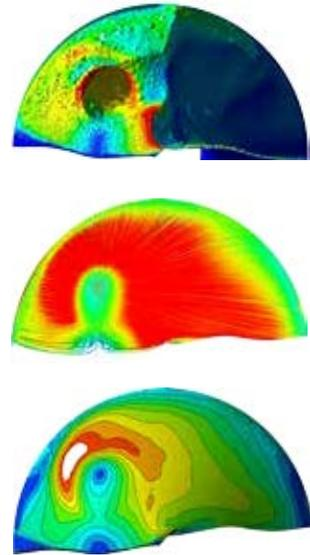
▲ End view of cutting area showing velocity contours of the coolant on the cutting tool surface (top), streamlines (middle) and velocity contours on the bore surface (bottom).
