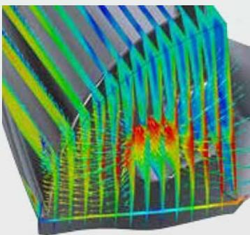
▲ End view of vertical plane showing the coolant velocity vectors
