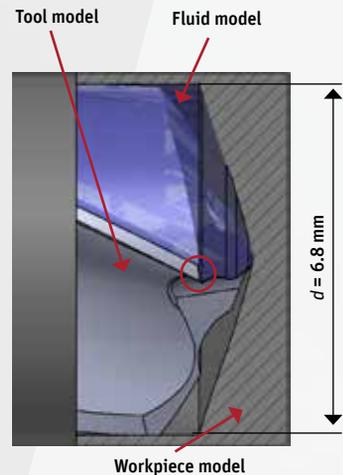
▲ Close-up view of cutting edge, including the solid tool zone, fluid zone and Inconel 718 solid workpiece zone
