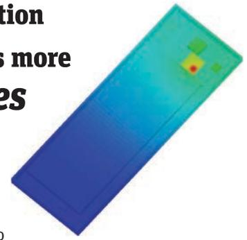
processor. A system-level thermal simulation produced nine outputs corresponding to the junction temperature of all the processors and sensors in the smartphone: one output each for the four main processors; three outputs for the dedicated processor; and two outputs for the two sensors on the chip.
