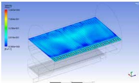
▲ Velocity profile over horizontal cross-section for the final smoker design. The final design has one long skinny inlet on the bottom and one long skinny outlet at the back angled at 30 degrees upward.
