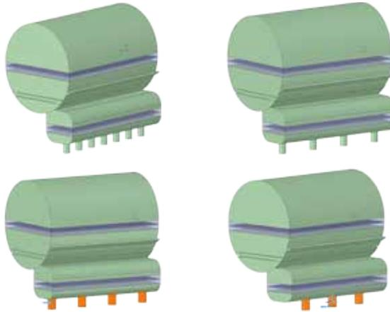
▲ Jacobs Analytics digitally explored many designs before determining the best configurations. Only a portion of the designs for the number and shape of inlets is shown.
