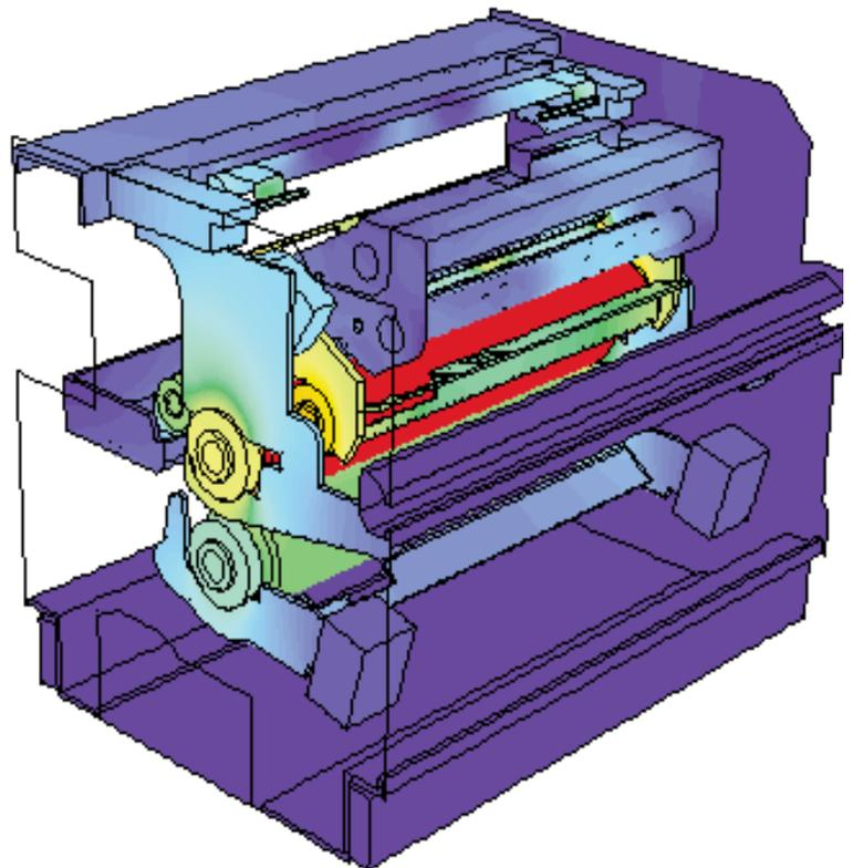
Figure 1: Temperature distribution of the fuser system viewed from paper exit. (Some components removed for clarity.)
