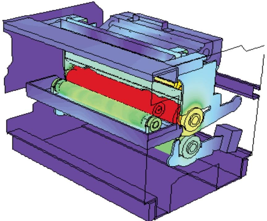
Figure 2: Temperature distribution of the fuser system viewed from the paper entrance. (Some components removed for clarity.)
