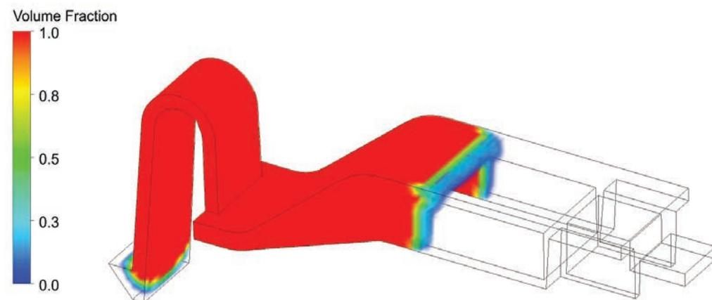
Volume fraction of plastic filling the mold
