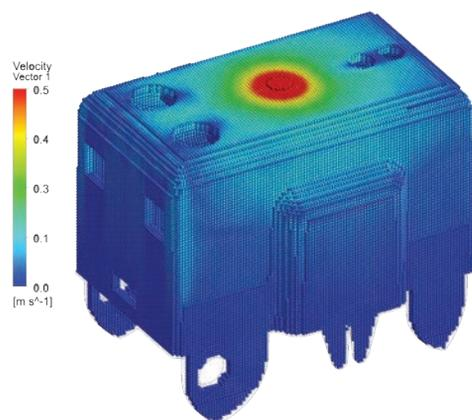
Velocity vectors of the plastic filling the mold
