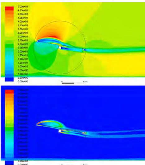
A vortex forms along the upper side of the panel during the simulation at 0.30 seconds.
