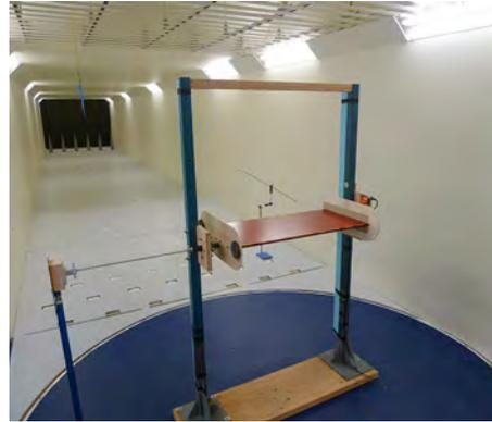
Model used for wind tunnel testing
