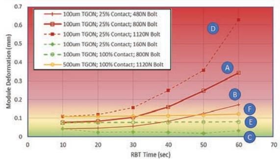
Nonlinear buckling analysis results with area colored red indicating cracking failure and area colored green indicating no cracking. Case C has little deformation but fails due to solder remelting. Case E has little deformation and a low temperature but could not be produced with the existing manufacturing process. Case F provides acceptable levels of deformation and temperature, but with no margin of safety, so even small levels of manufacturing variation could cause failures.
