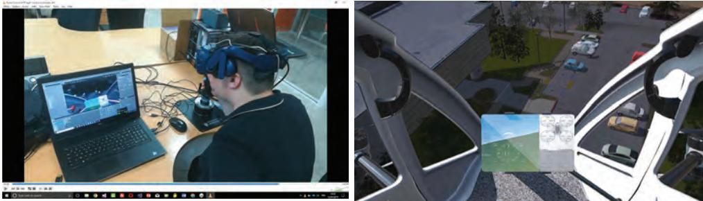
The ANSYS VRXPERIENCE platform enables engineers to test the impact of a specific control law – developed with the SCADE software suite – on the real-world human experience. The simulation user is fully immersed in a highly accurate virtual reality environment, and can experience a complete VTOL flight scenario long before the real aircraft exists.
