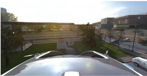
Vertical takeoff of a drone in an urban environment. Since vertical takeoff is driven by the output of camera sensors installed on the drone, it is crucial that these sensors are simulated and tested for reliable performance.
