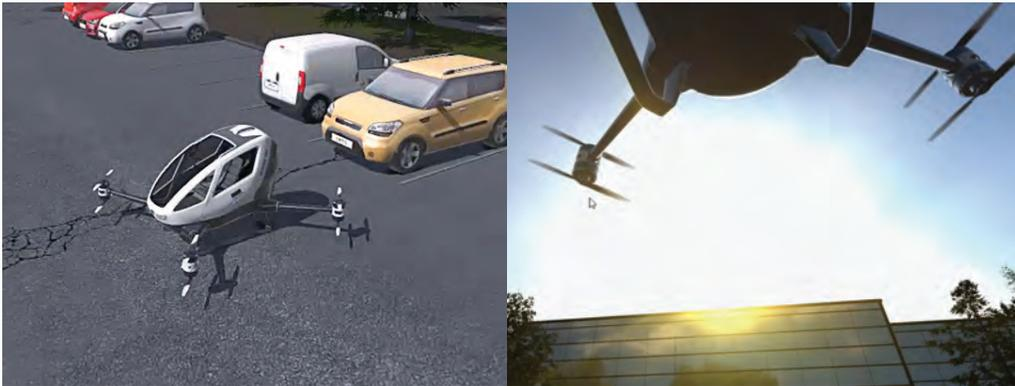
This ANSYS simulation of a drone in an urban virtual environment includes physical factors such as the effects of wind on flight dynamics, and accounts for optical phenomena such as the reflection of sunlight on glass buildings.
