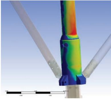
▲ Structural analysis of 40E airship landing gear reveals the most critical stress areas under a range of landing conditions.
