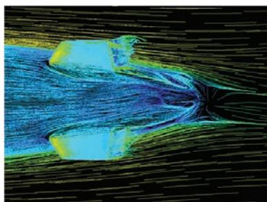
▲ CFD simulation of 40E airship shows turbulent behavior on control surfaces and the wake behind the airship.
