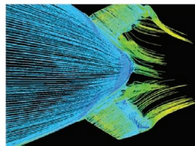
▲ CFD simulation of 40E airship demonstrates the effects of ruddervator (combined rudder and elevator) angle of attack and deflected airstream.
