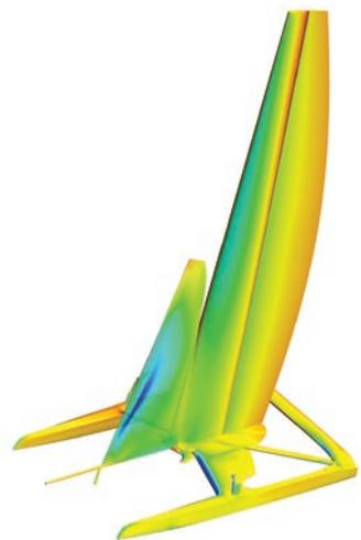
▲ Use of engineering simulation helped ETNZ to improve yacht aerodynamic performance in both downwind (top) and upwind (bottom) conditions.
