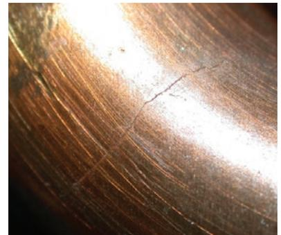
▲ Example of fatigue failure
