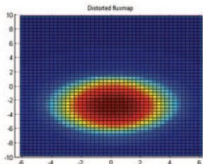
▲ A MATLAB routine converted deformation into flux maps that show energy reaching receiver in tower. An ideal flux map (top) is produced by a perfectly stiff structure; flux map on bottom shows a more realistic case.
