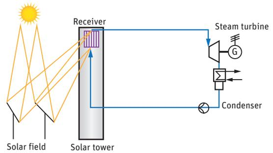
▲ Operation of power tower CSP plant shows how heliostats focus light on a central receiver that transfers heat to a fluid that, in turn, produces steam.
