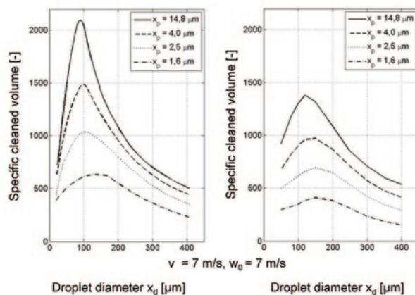
▲ ANSYS CFX numerical modeling results (right) matched Löffler's theoretical calculations and experimental data (left).
