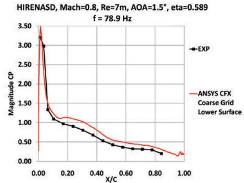
▲ Simulation predictions of unsteady-state coefficient of pressure for HIRENASD correlate well to wind tunnel experiments.
