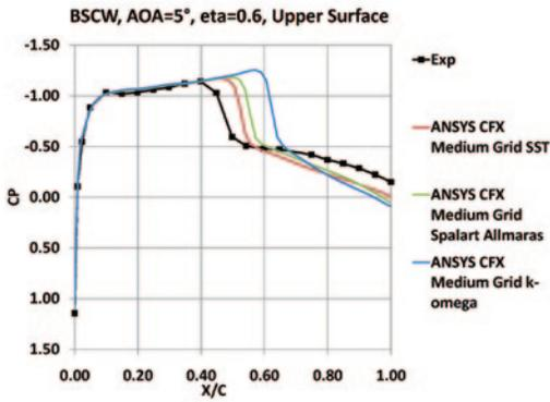
▲ ANSYS CFX turbulence model error for BSCW at steady-state conditions
