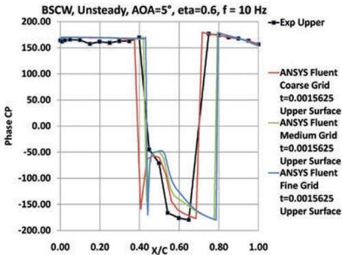
▲ Fluent calculations for BSCW show good fit with experimental measurements.
