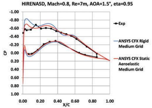
▲ Comparison of static aeroelastic equilibrium simulation predictions to experimental measurements for HIRENASD
