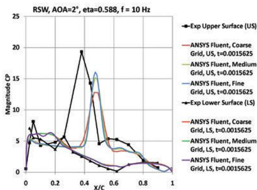
▲ Comparison of ANSYS Fluent CFD results to wind tunnel experiment for RSW dynamic test case at 10 Hz
