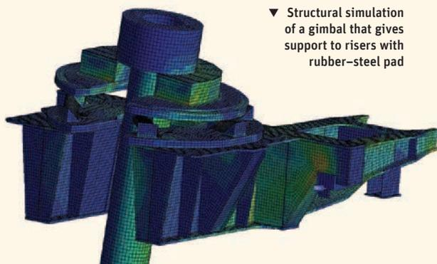
▼ Structural simulation of a gimbal that gives support to risers with rubber-steel pad
