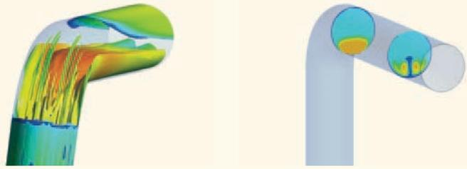
▲ Frequency fluctuations downstream of single pipe bend
