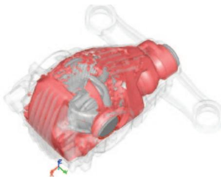
Oil distribution calculated with CFD using VOF model to identify free surfaces
