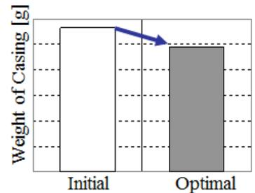
Design changes made with input from CFD simulation maintained the existing optimal oil temperature while significantly reducing case weight.
