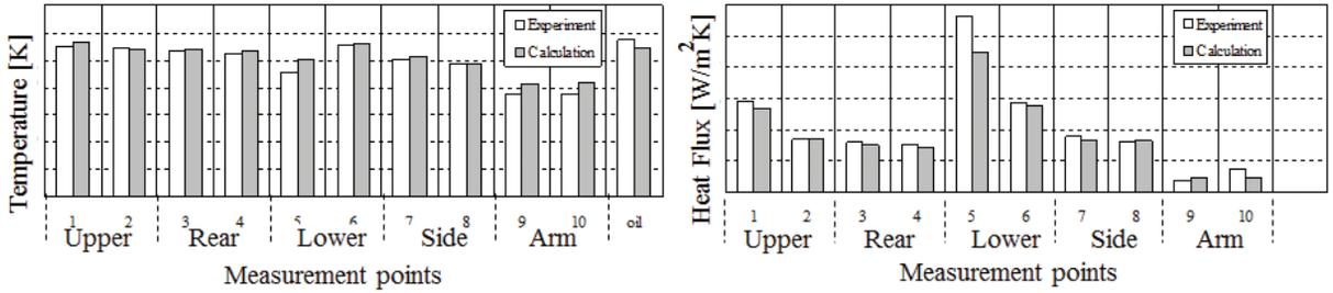
Heat calculation model generated predictions of heat flux distribution and temperatures, which agreed well with measurements.
