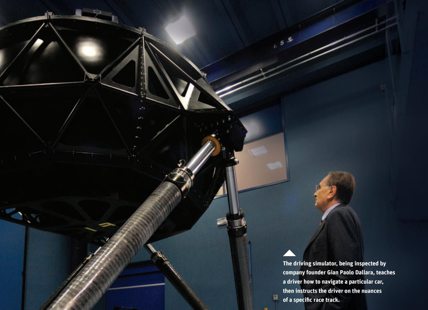
▲ The driving simulator, being inspected by company founder Gian Paolo Dallara, teaches a driver how to navigate a particular car, then instructs the driver on the nuances of a specific race track.
