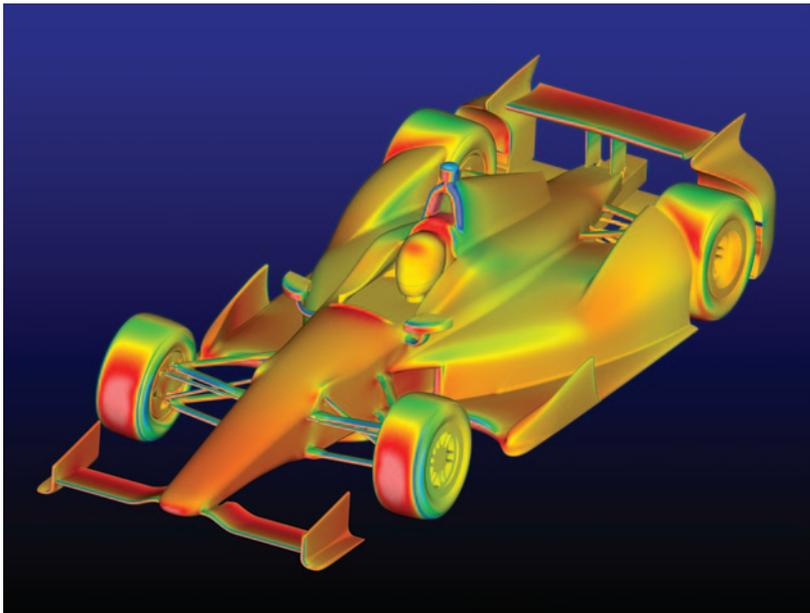
▲ ANSYS CFD allows Dallara to perform the simulations required and to link with structural analysis data. Pressure contours for the 2012 Indy car were generated using ANSYS Fluent software.
