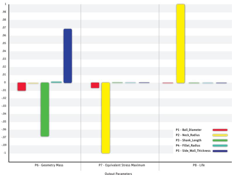
**Fatigue life optimization based on neck radius for a trailer hitch**
