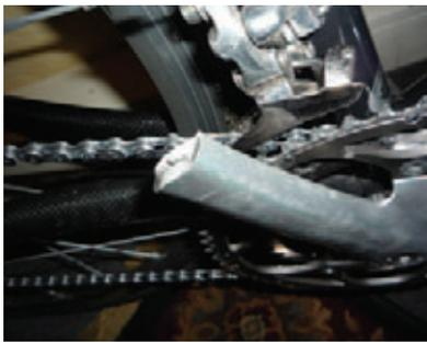
**Bicycle crank fatigue failure from cyclic loading**
