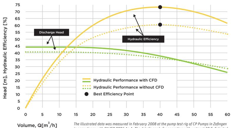
The illustrated data was measured in February 2008 at the pump test rig of CP Pumps in Zofingen in accordance with EN ISO 9906 An.A. The details apply for operation with water at 20 C. Selected pump: MKP 65-40-160 with impeller diameter 180 mm at 2930 mi n-1.
