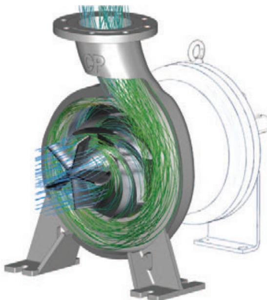
engineers to quickly and easily model impeller geometries. This tool enables the user to design both the meridional flow path and the blade shape, including the blade-thickness distribution. Once blade geometry is specified, the software determines the cross-sectional area along the flow path to enable assessment of flow characteristics.
