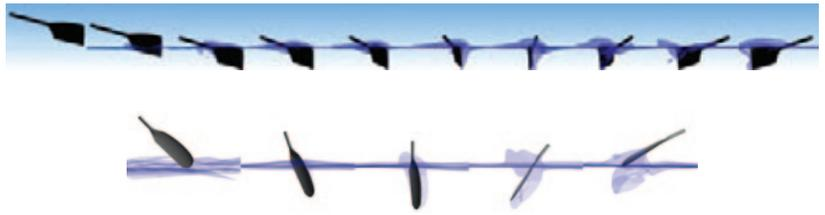
Sequence of blade stroke as the blade contacts water: rowing oar (top); kayak paddle (bottom)
