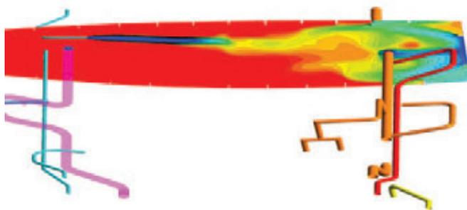
Result from wing tank ullage space CFD analysis showing instantaneous oxygen concentration contour lines in a “spar” plane through the center of a nozzle injecting nitrogen-enriched air into ullage space for inerting purposes.
