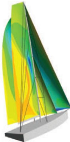
▲ **The CFD simulations included sails, boom, mast and approximate hull geometry. CFD results allowed the team to model rigging windage by sampling velocities at discrete locations along each rigging element — and then pinning these elements to the CFD geometry.**
