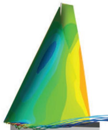
**Physical tests in a twisted-flow wind tunnel produced images that seeded subsequent CFD simulations of sail performance.**
