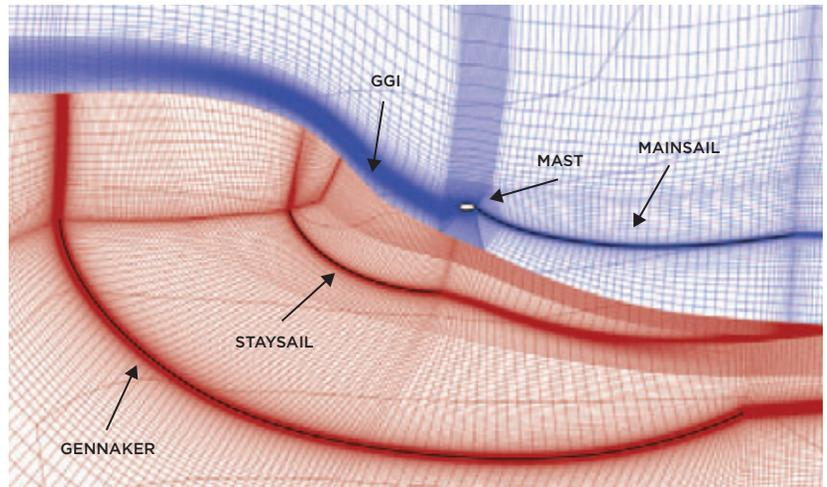
▲ **Block-structured grids of the sails generated based on images from wind-tunnel tests. To retain high-quality cells and a simple blocking topology, Emirates Team New Zealand engineers made use of generalized grid interfaces (GGIs).**
