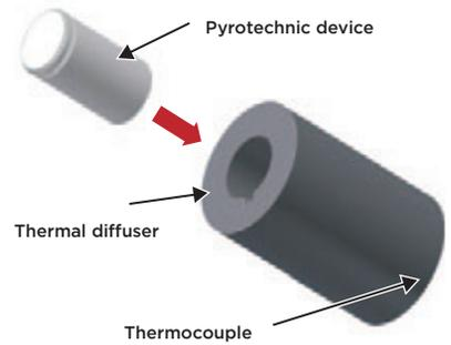
After receiving an electrical signal, the fusehead ignites an energetic redox material.
