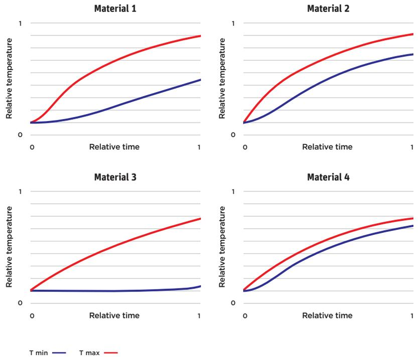
Thermal diffuser maximum (red) and minimum (blue) temperatures as a function of time. The objective was to minimize the difference between the two to heat the largest possible volume of material. Materials 2 and 4 had good thermal properties. Material 2 was selected because of its superior machinability.
