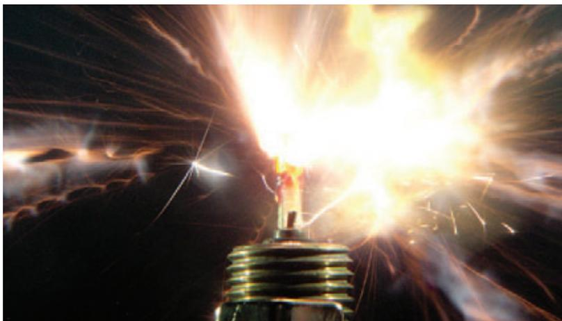
Fusehead of a small pyrotechnic device
